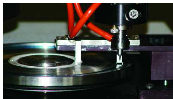
Multiple epoxies with multiple stamping tools enable stamping of a large variety of materials and dot sizes
