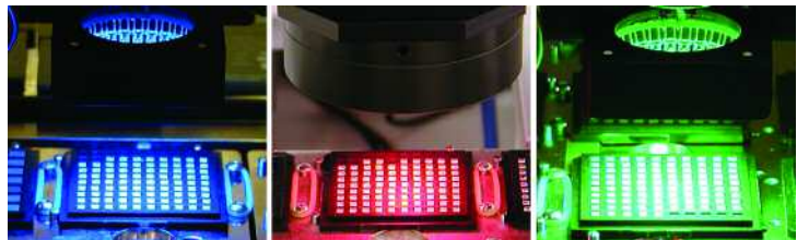
Blue, red and green programmable lighting for vision processing of challenging substrate materials
