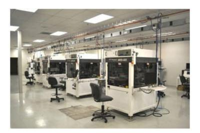
As the needs for greater accuracy increase the demand for in-situ UV curing also increases. UV curing during assembly provides the advantage of eliminating post bond cure movement. Our die bonders are available with a wide range of UV dispensing and curing options including integrated automatic material handling.
